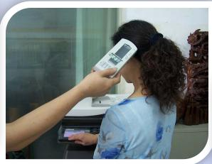
接觸影印機後,人體腦部電磁波量測值達238V/m
